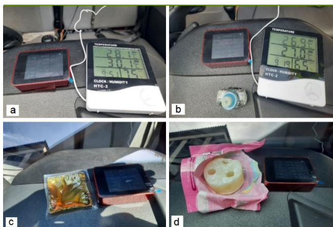
Figure 4. Experimental conditions: (a) control without air freshener, (b) liquid air freshener, (c) gel air freshener, and (d) solid air freshener
