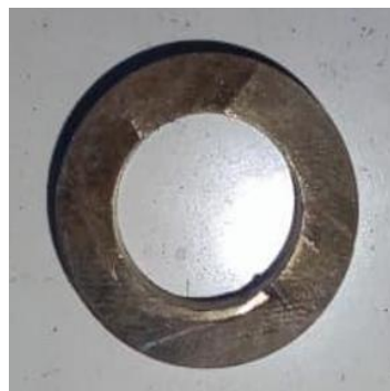
Figure 3. Replacement bushing for the starter gear
