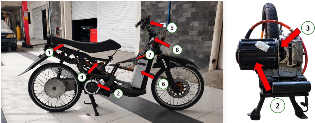
Figure 7. Photographic view of the electric-motor installation on the Yamaha 5TL frame (1. Yamaha 5TL frame, 2. BLDC motor, 3. Bracket, 4. ECU, 5. Hand throttle, 6. Battery, 7. MCB, 8. Ignition switch)
