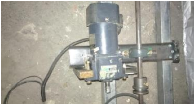
Figure 4. AC gear motor used to drive the open-close mechanism.
