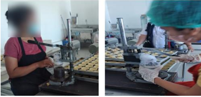
Figure 2. Manual dough-forming process for milk pie: (a) placement and shaping of the dough in the mold and (b) pressing of the dough by the operator
